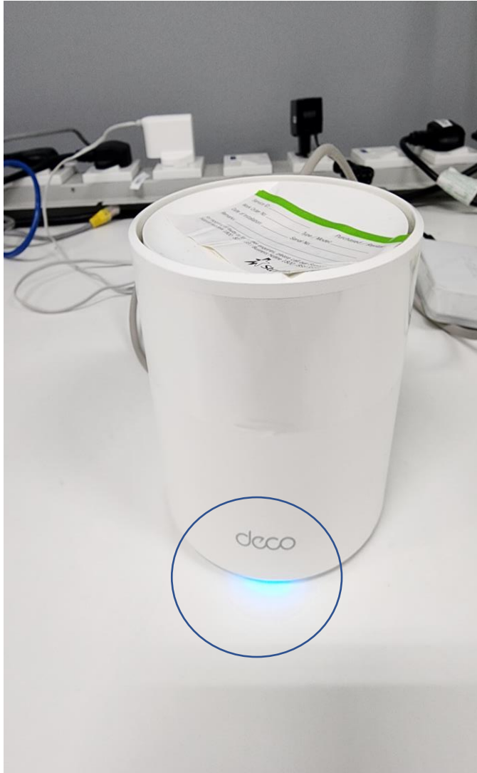
Installation In Progress (blue)
