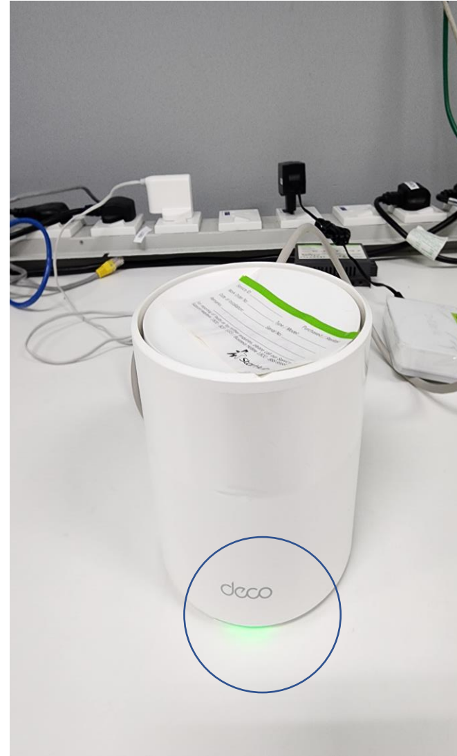
Installation Completed (green)
