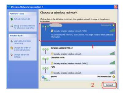
3. Input WiFi Key in the dialog of password input then click to establish connection(The WiFi Key and the SSID can be found on a label stick inside the back cover)
